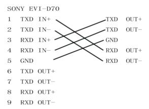
The following picture shows the RS485 wiring diagram of KT-HD61C camera and K1:
